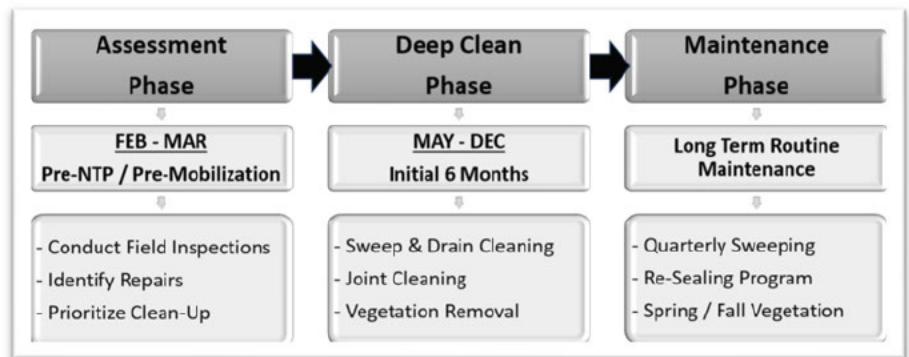
Figure 20 - AIMM's Bridge cleanup approach
